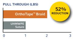
Force Fiber® OrthoTape $^{TM}$  Braid won't pull through as easily as a round suture.\*\*
